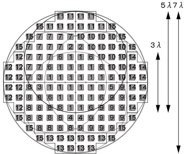
Fig.3 Transducer array elements of the J-QUEST transducer. Transducer channel diameters are indicated using wavelength ( $\lambda$ ).
