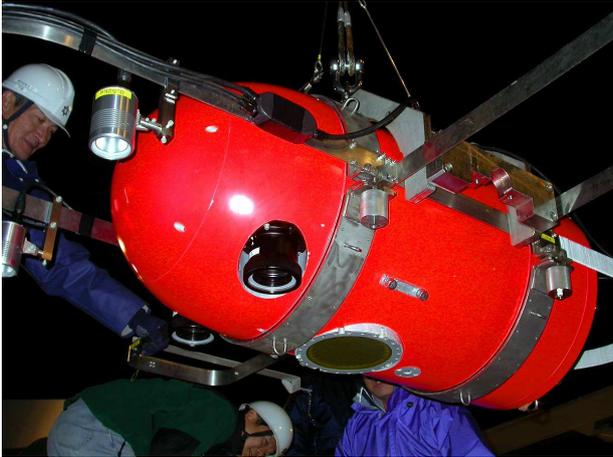
Fig.1 Tethered J-QUEST on deck.
