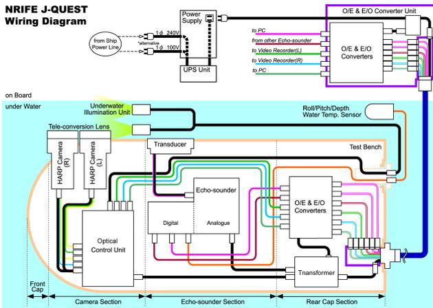
Fig.2 J-QUEST system block diagram
